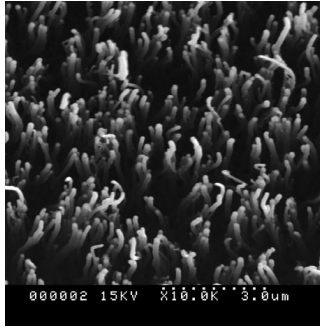
Figure 1: SEM image showing randomly oriented tips of CNTs in a thin film.
