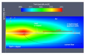
As an example we present simulation results of a GaN pin-diode with three embedded In<sub>0:05</sub>Ga<sub>0:95</sub>N QW, including an AlInN oxidization layer for current focusing. The heat transport simulation includes the air around the device, whereas the particle transport simulation is limited to the semiconductor. In Figure we show the temperature map at a bias voltage of 5.1 V, which corresponds to a current of
